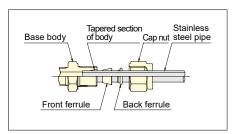
Confirm whether the parts of a base fit as shown in the figure above, and then insert a stainless steel tube until its end makes contact with the back of the body.
