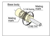
From this position, tighten the cap nut by turning it one and one-quarter turns with a wrench.
