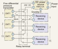
This DC power unit <HWS15A> can supply 24 V DC power to up to 15 two-wire type fine differential pressure transmitters. Provide relay terminals for DC power distribution use as shown in the figure above, and supply power to each transmitter. The user should prepare the relay terminals for distribution use.
